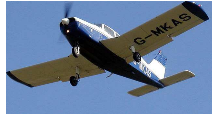
Low aspect ratio wing (AR=5.6) of a
